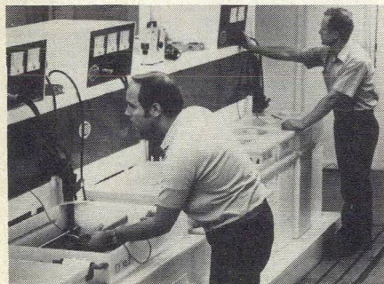
4. Electro-forming process at Gamma-F Corporation uses an electrolytic bath of copper sulfate to plate precision components onto a mandrel.
